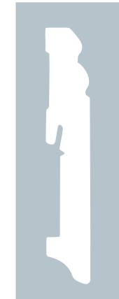
Skirting board 18/115 MDF material 18 x 115 x 2400 mm VE = 4 units
