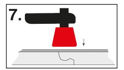
Gently tap with a rubber mallet and make sure the plates are locked.
