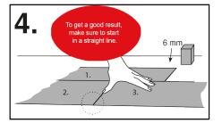
Press the short end of the tile straight down. Leave a 6 mm gap (movement joint) against the wall around
