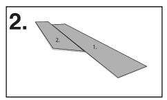
Start by clicking two long sides together. Use a laying tool to get the right angle when the tiles are clicked together.
