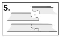
Clarifying picture of how the short end of the plate should be pressed straight down.
